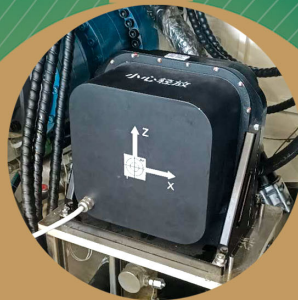
慣性導航系統及里程錶 Inertial Navigation System and Odometer
